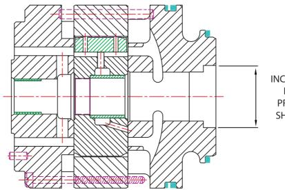
INCREASED OPENING AND DEPTH DIMENSIONS PROVIDING INCREASED SHAFT HUB CLEARANCE
