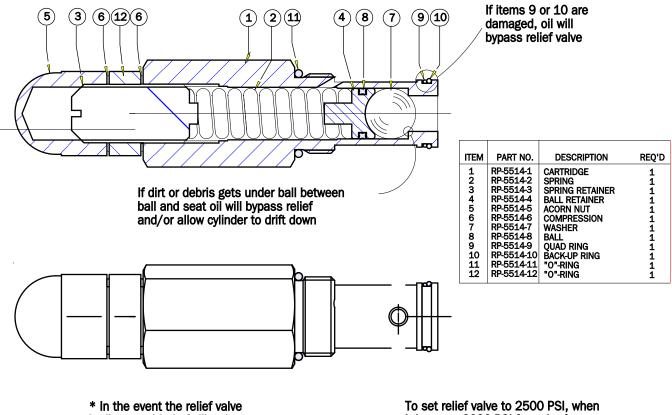
is disassembled - Calibration must be done on a test stand it is set at 2000 PSI from the factory remove item #5, loosen item #12, turn item #3 3/8 of a turn clockwise then tighten item #12 and replace item #5.
